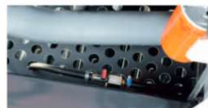
Fuel tank water drainage cock
