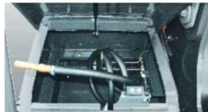
Electric fuel refilling pump
